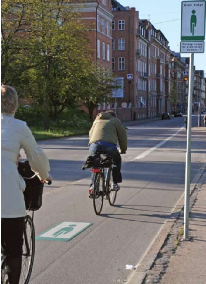
Figure 32. “Green wave” cycle track in Copenhagen, Denmark, on which traffic signals are synchronized to bicyclist speeds.
